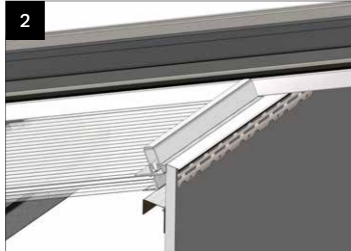
Ultraframe supplies a plasterers stop bead (CHA300) for the top edge adjacent to the glazing – ensure it is attached as shown. Be careful when handling/cutting this item not to damage the paint surface.
