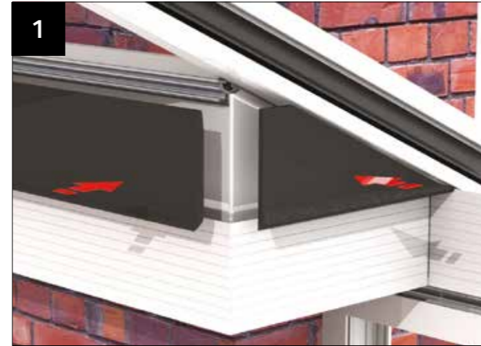
If not already fitted, attach box gutter insulation foam to the upper section of box gutter.
