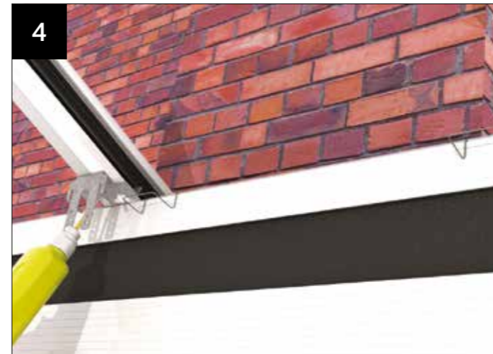
Fit brackets in marked positions on the bars as per standard installation
